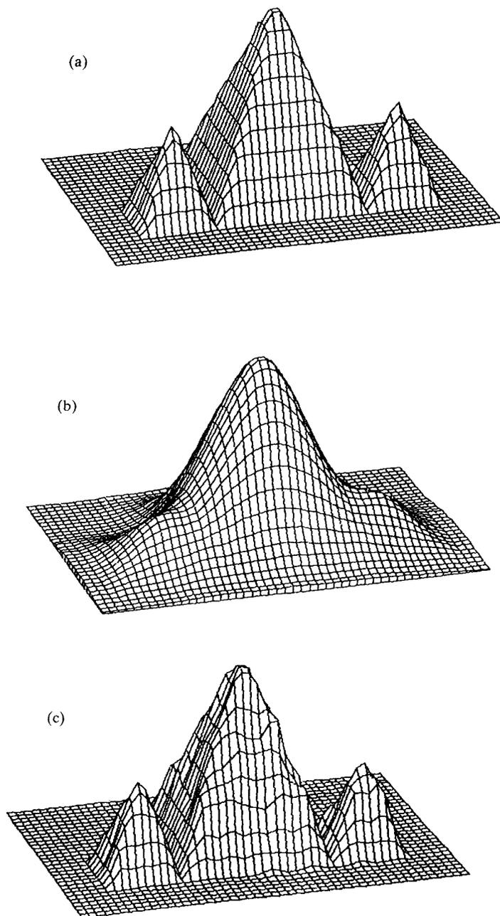
**Figure 5** Test object (a), degraded due to smoothing and external noise image (b) and the MLIR-estimate with non-negativity as a sole *a priori* information (c).
