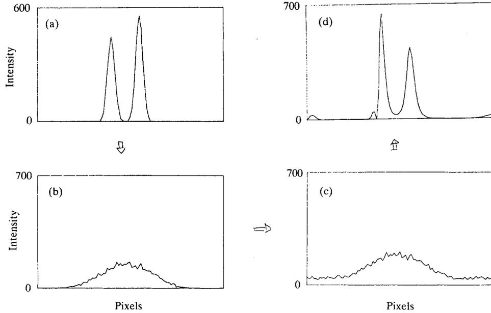
**Figure 1** Example of blurring and restoring of an object; a—initial image (object), b—result of stochastic smoothing by an imaging system, c—observed image after adding external noise to previous image, d—result of restoration with the aid of MLIR method.
