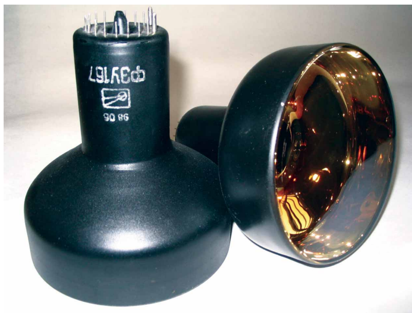
Figure 4. FEU-167 and FEU-167-1 PM tubes. The photocathode section diameter is 125–130 mm.
