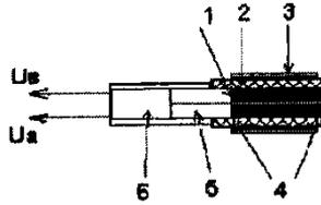
FIGURE 7 The construction of the EPHOS detector consisting of four  $\text{PbWO}_4$  crystals: 1,  $\text{PbWO}_4$  crystals; 2, copper heat exchanger; 3, cooling element; 4, temperature-sensing elements; 5, photomultiplier-175; 6, photomultiplier dividers.
