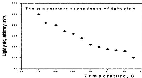
FIGURE 5 The temperature dependence of the  $\text{PbWO}_4$  light yield.
