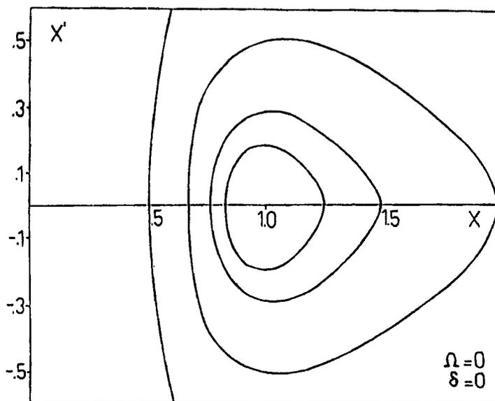
Figure 2 Phase diagram for  $\Omega = 0$  (i.e. no radiation). All trajectories are stable oscillations.
