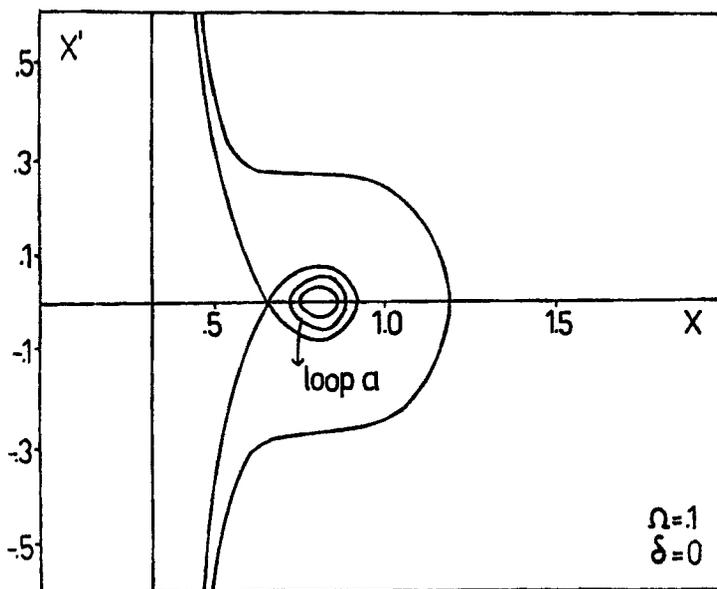
Figure 3 Phase diagram for  $\Omega = 0, 1$  (i.e.  $\Omega < \Omega_c = 0, 10$ ). There are two singular points  $x^+$  and  $x^-$ . For  $0, 67 < 0, 92$  the oscillations may occur. For  $x$  outside this interval the shell always collapse.
