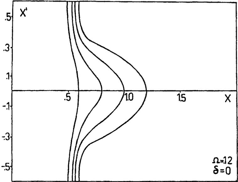
Figure 4 Phase diagram for  $\Omega = 0,12$  (i.e.  $\Omega > \Omega_c = 0,10$ ). There are no singular points. All trajectories yield the shell collapse.
