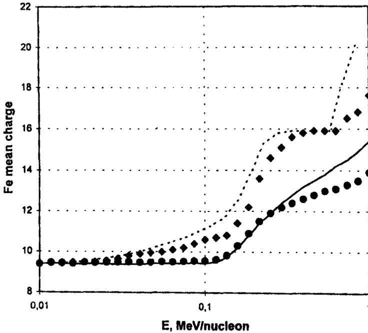
**Figure 4** The mean charge of accelerated Fe ions simulated for  $\tau = 1.6$ ,  $S = 5/3$ ,  $T = 10^6$  K and  $NT_{ac}^q$  (at 10 MeV nucleon $^{-1}$ ) =  $(1.2-0.8) \times 10^{10}$  s cm $^{-3}$ . Dashed curve is the equilibrium Fe charge, solid line – the Monte-Carlo stationary solution (see text), circles and rhombs are the Monte-Carlo solutions for the particle population escaping the downstream boundary  $x_{max} = 94D_{02}/u_2$  and  $x_{max} = 625D_{02}/u_2$ , respectively.
