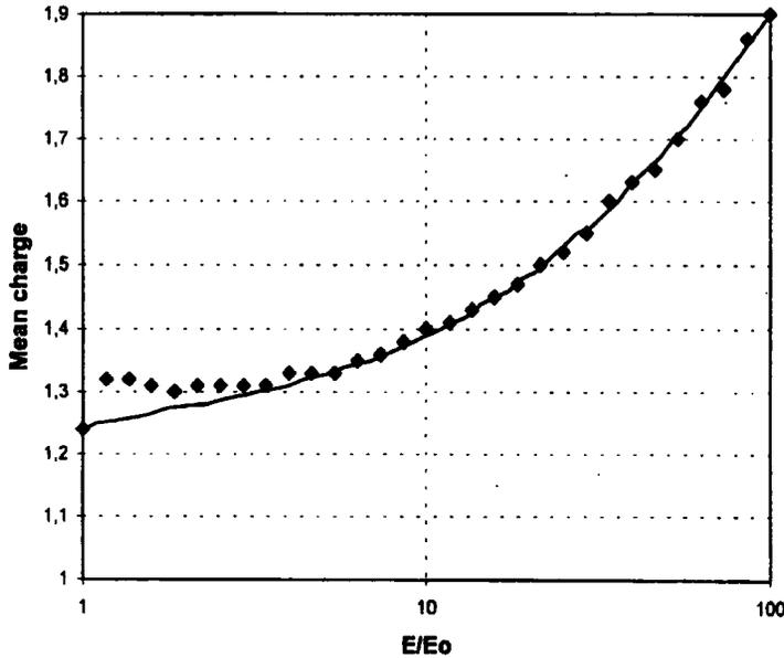
**Figure 1** Energy dependence of the mean charge of accelerated ions (three-level model) simulated both by Monte-Carlo (rhombs) and by finite differences (solid line) methods for  $r = 1.6$ ,  $S = 5/3$ ,  $T_{ac}^{+2}/T_{ac}^{+1} = 0.8$ ,  $T_{ac}^{+3}/T_{ac}^{+1} = 0.7$ ,  $\tau_{12}/T_{ac}^{+1} = 0.7$ ,  $\tau_{23}/T_{ac}^{+1} = 1.4$ ,  $\tau_{10}/T_{ac}^{+1} = 10$ , and  $\tau_{21}/T_{ac}^{+1} = \tau_{32}/T_{ac}^{+1} = 8.6$  at  $E = 100E_0$ .
