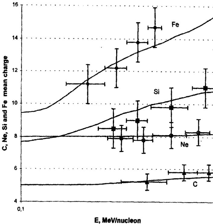
**Figure 3** The mean charge of accelerated Fe, Si, Ne and C ions simulated for  $r = 1.6$ ,  $S = 5/3$  and  $T = 10^6$  K; for iron  $NT_{ac}^q = (1.2-0.8) \times 10^{10}$  s cm $^{-3}$ , for silicon, neon and carbon  $NT_{ac}^q = (0.9-0.8) \times 10^{10}$  s cm $^{-3}$  (at 10 MeV nucleon $^{-1}$ ). Also shown are the observations from the ACE spacecraft for the 6 November 1997 SEP event (Möbius *et al.*, 1999).
