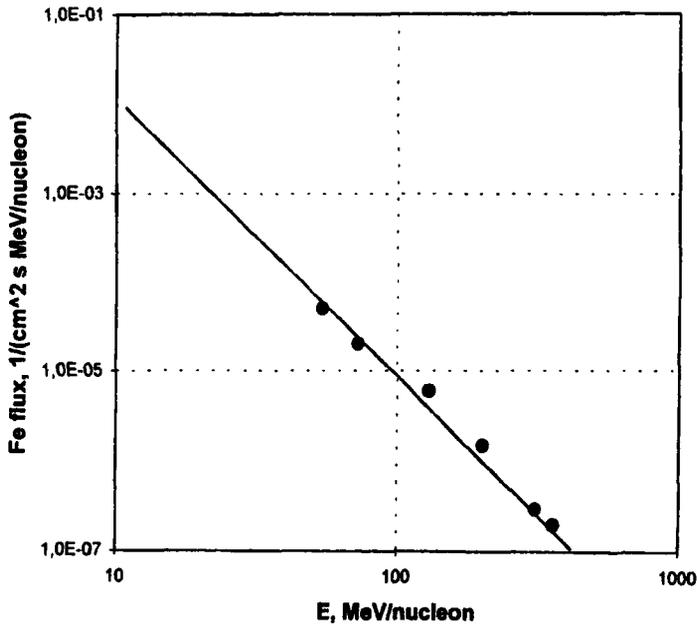
**Figure 2** Fitting of the Fe flux summed over all charge states simulated for  $r = 1.6$ ,  $S = 5/3$ ; circles - experimental data from the IMP-8 satellite for the 6 November 1997 SEP event.
