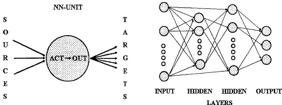
**Figure 4** Artificial neural network structure. Left: a unit (neuron) and its functions; right: the ANN layers.
