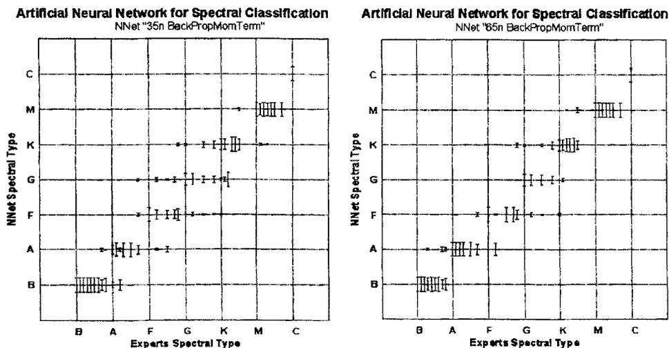
**Figure 6** The artificial neural network classifications vs. expert spectral types (the vertical bars show the classification weights). Left: ANN trained with 35 patterns; right: ANN trained with 65 patterns.
