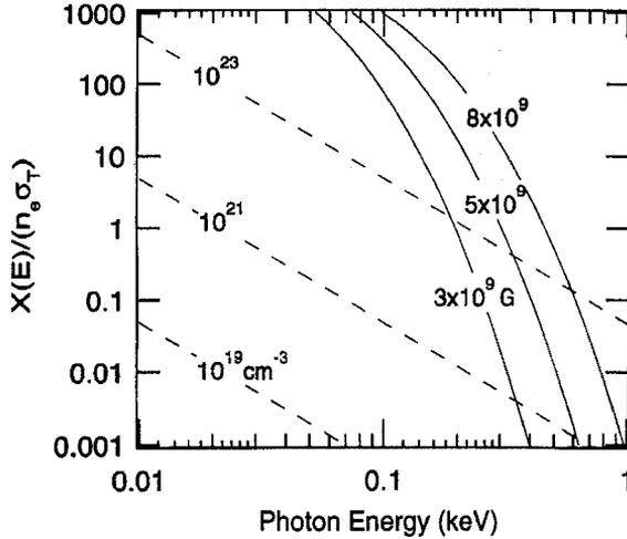
**Figure 1** Coefficients, in units of the coefficient for electron scattering, for cyclotron absorption (solid lines) and inverse thermal bremsstrahlung (dashed lines), for an electron temperature of 10 keV and several magnetic field strengths and electron densities.
