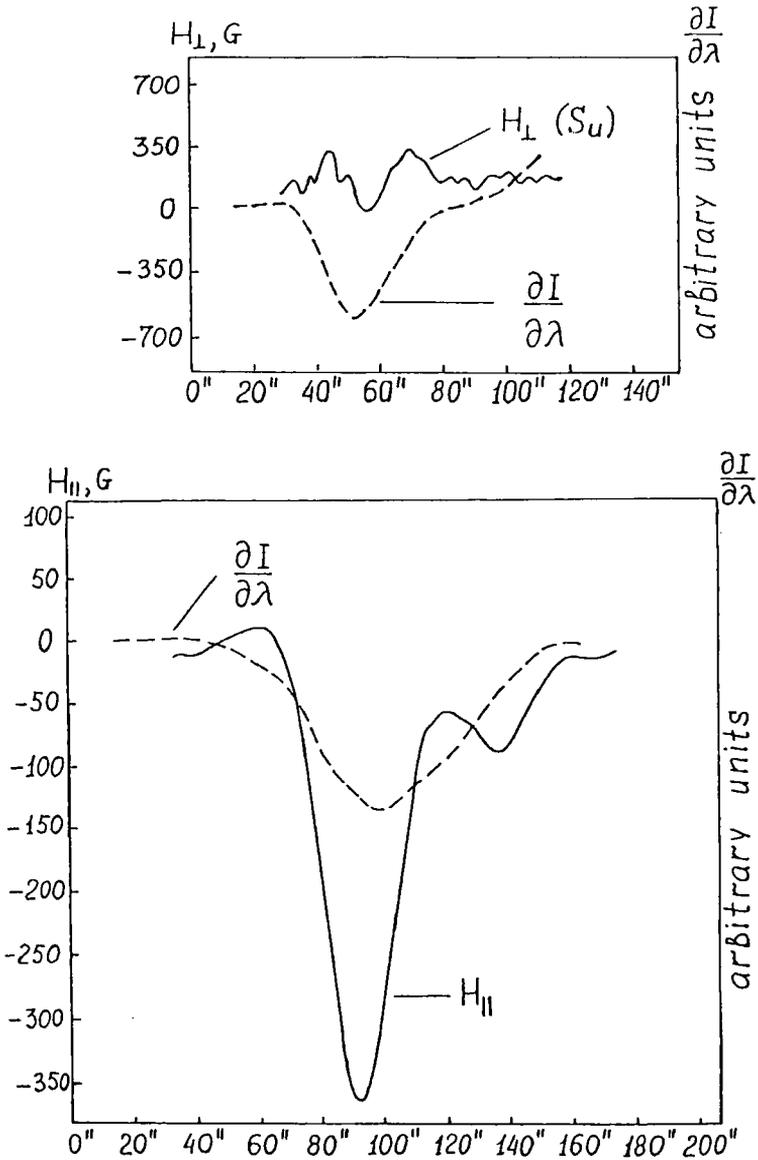
**Figure 3** Fragments of scans in the line FeII 6149.2Å; entrance aperture 8" x 1.5". Top: scan through a plage area at the limb. Bottom: scan through an active region.
