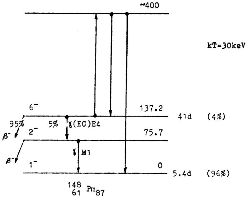
**Figure 3** Level scheme of  $^{148}\text{Pm}$  with conventional level at 400 keV which permits the equilibration of the ground and isomeric  $^{148}\text{Pm}$  states. Lesko *et al.* (1989) have identified three such levels at  $\approx 400$  keV.
