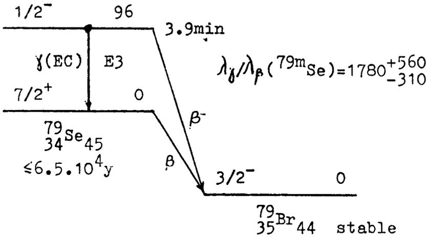
Figure 4 Decay scheme of  $^{79}\text{Se}^{g,m}$  with the allowed  $\beta^-$ -transition for  $^{79\text{m}}\text{Se}$  ( $1/2^- \rightarrow 3/2^-$ ) the probability of which has measured by Klay and Käppeler (1988).
