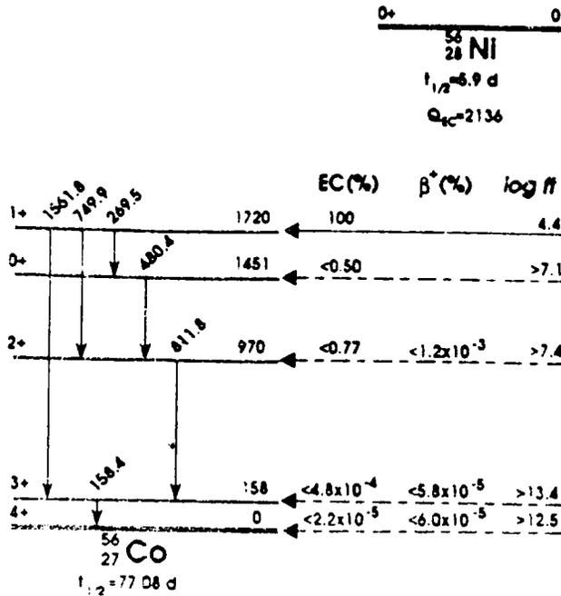
Figure 2 Decay scheme for <sup>56</sup>Ni showing EC and  $\beta^+$  branching ratios measured by Sur *et al.* (1990) (Figure 1 in their paper).
