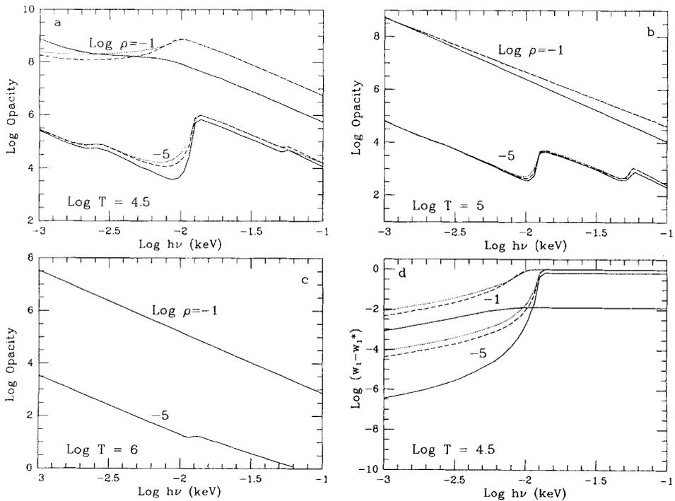
**Figure 2** Opacity spectra (a, b, c) and microfield jump smoothing factor  $W_i - W_i^*$  (d) of Lyman-hydrogen ionization jump for the H–He mixture corresponding to Figure 1 at  $\rho = 10^{-1}$  and  $10^{-5}$  g/cm<sup>3</sup>. Solid, dashed and dotted curves have the same meaning as in Figure 1.
