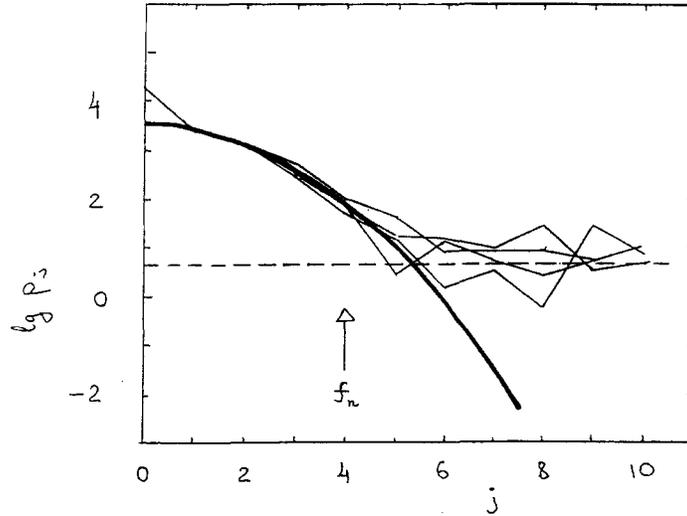
**Figure 5** The power spectra for deterministic Gaussian object (thick line), background (dotted line), and four random simulations of the noisy Gaussian object.
