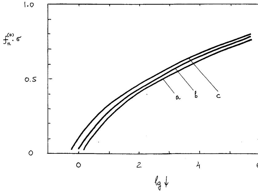
**Figure 6** Relation between the noise-limit frequency  $f_n^{(0)}$  and signal-to-noise ratio for Gaussian stochastic object;  $\alpha = 0.10, \beta = 0.05$  (a),  $\alpha = \beta = 0.20$  (b),  $\alpha = \beta = 0.30$  (c).
