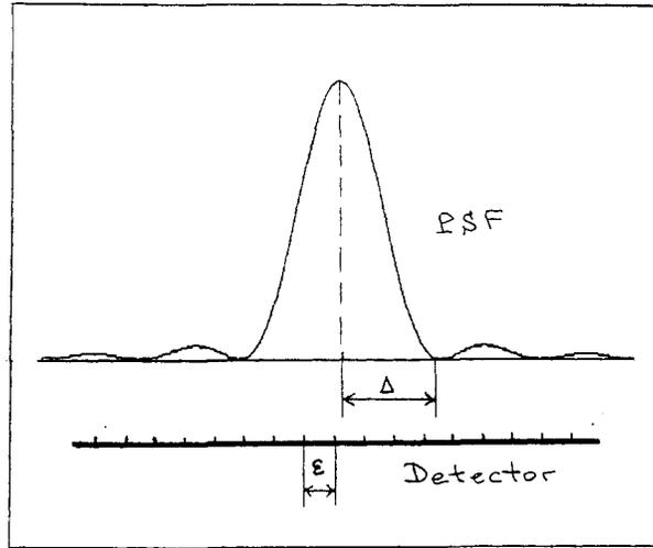
**Figure 1** Schematic representation of the Point Spread Function width  $\Delta$  and detector pixel size  $\epsilon$ .
