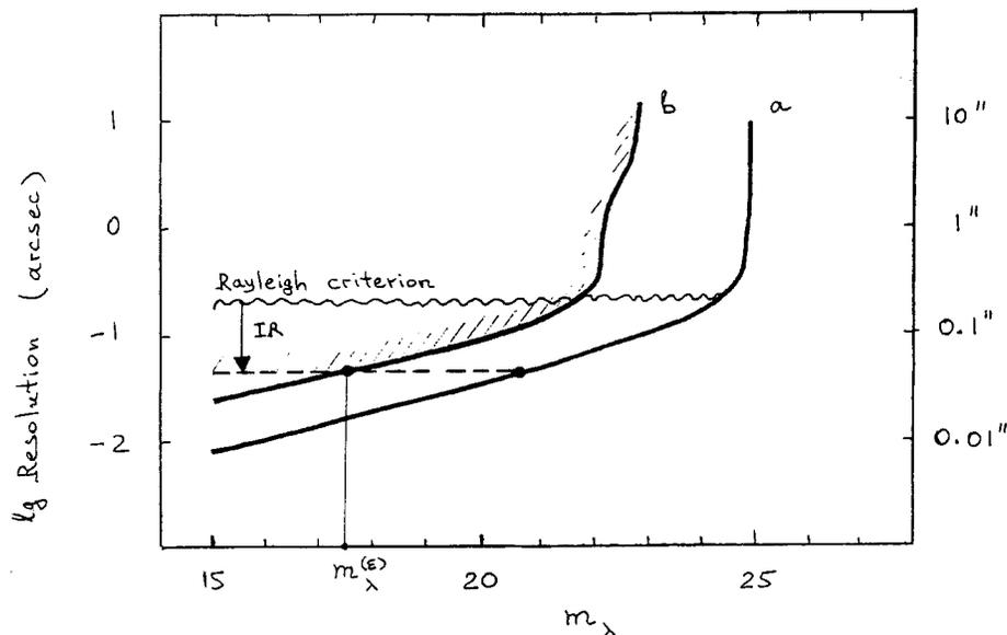
**Figure 8** The resolution-magnitude relation for  $f/96$  FOC HST images under the conditions specified in Table 3. Thick lines correspond to the theoretical limit for the supposed (a) and real (b) HST optics wavy line corresponds to the Rayleigh law and dashed line shows the resolution limit due to the pixel size. The shaded area is accessible for the actual HST optics. The symbols "IR" indicate the image restoration techniques abilities.
