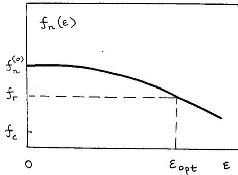
**Figure 7** Qualitative form of the relation between the noise-limit frequency  $f_n$  and pixel size  $\epsilon$ .
