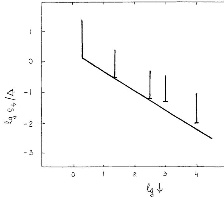
**Figure 3** Theoretically minimum resolution  $\rho_t$ , as a function of signal-to-noise ratio for the choice of objects (solid line) and results of numerical simulations for non-negativity as the only *a priori* information (vertical bars).
